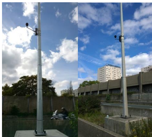
Figure 1 Permanent noise measurement stations installed by Bruitparif since early September 2017 on the A6 motorway at L'Haÿ-les-Roses.
